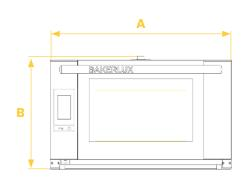
Oven must be min. 2" from the wall on both sides (left and right).
